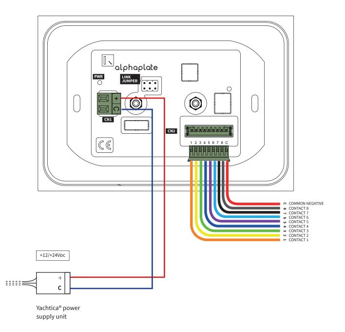
**PWR:** Led power supply on If properly connected, green light on **CN1:** Power Supply Connector **CN2:** Contacts Wires Connector
