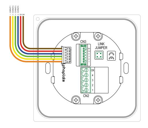
**CN2:** Connector for wiring insertion contacts
